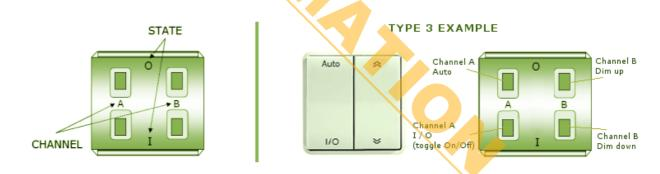
The button naming used below is referring to CHANNEL and STATE of the PTM200. Thus "Button Af" means STATE "I" on CHANNEL "A".
